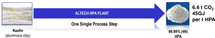
Figure 2 – Altech's Kaolin-Alumina Process
